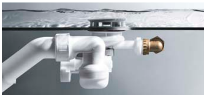
Multiplex Trio F for filling from the bathtub bottom up with electronic valve cone drive (connection to MT E-technology) Inlet, drainage and overflow fitting for bathtubs with 52 mm drain hole flat overflow with an installation depth of just 33 mm for particularly flat tub rims.
