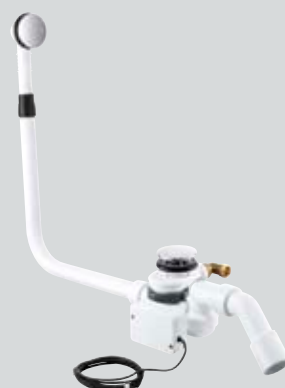
Multiplex Trio F for filling from the bathtub bottom up with electronic valve cone drive (connection to MT E-technology) Inlet, drainage and overflow fitting for bathtubs with 52 mm drain hole flat overflow with an installation depth of just 33 mm for particularly flat tub rims.
