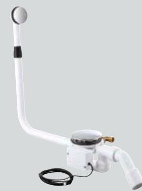
Rotaplex Trio F for filling from the bathtub bottom up with electronic valve cone drive (connection to MT E-technology) Inlet, drainage and overflow fitting for bathtubs with 90 mm drain hole flat drain hole with an installation depth of just 33 mm for particularly flat tub rims.
