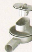
4982.93 Reconstruction model drain for installation heights from 70 mm, drainage capacity: 0.4–0.45 l/s, head water level: 25 mm
